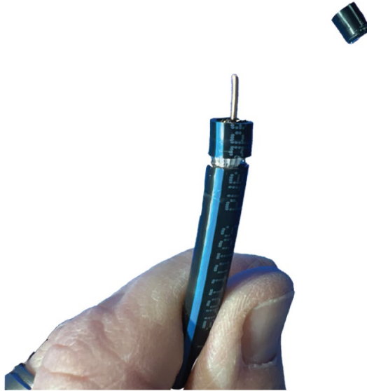
Figure 52: Exposing the center conductor
