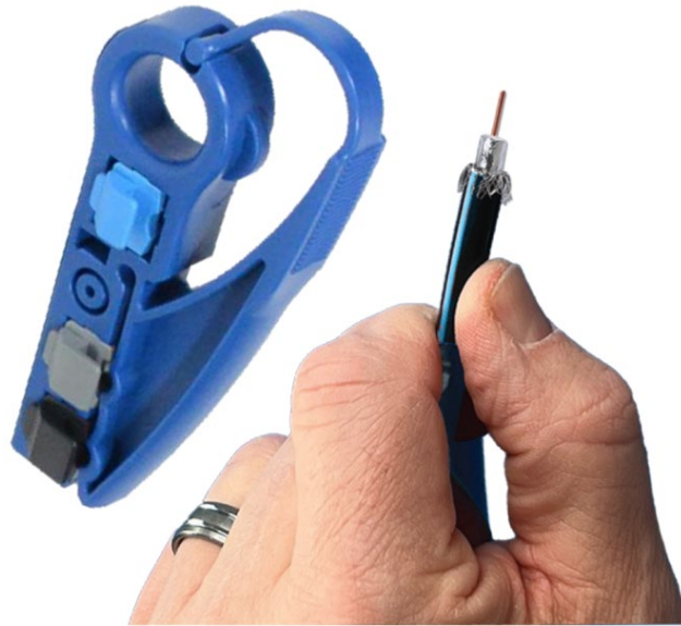
Figure 54: Folding the outer braid against the jacket
