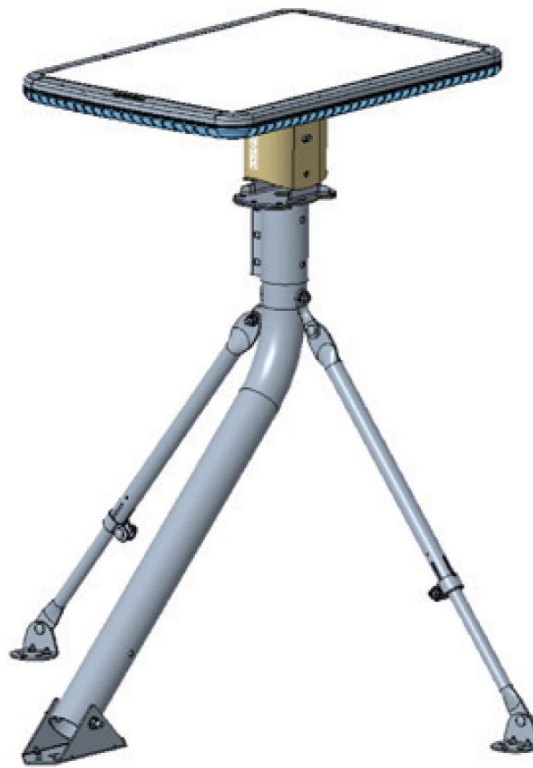
Figure 29: ODU Mounted to trimast mount with short stanchion
