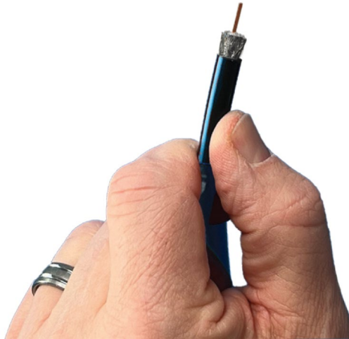
Figure 53: Exposing the braid and foil
