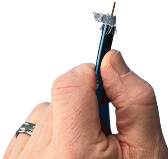
Figure 55: Cutting the inner foil
