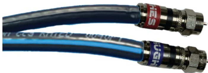
Figure 59: Finished IFL cables
