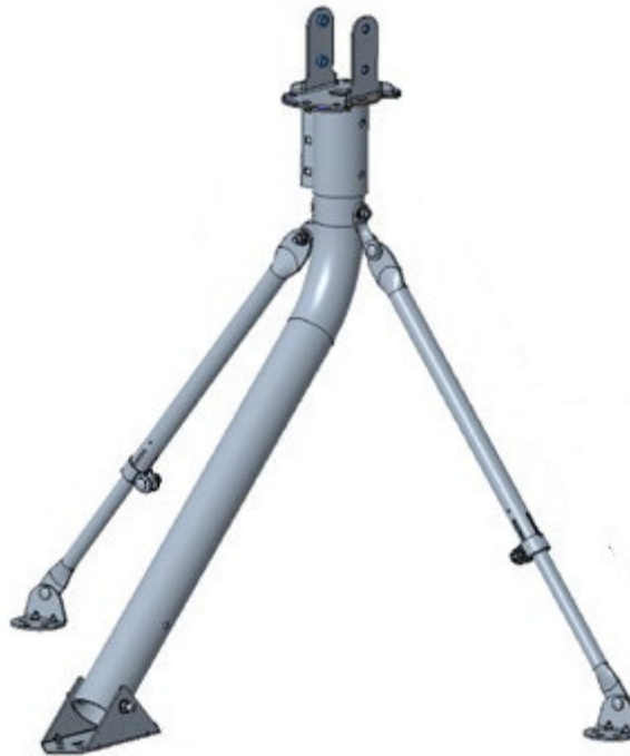
Figure 25: Mast adapter with trimast
