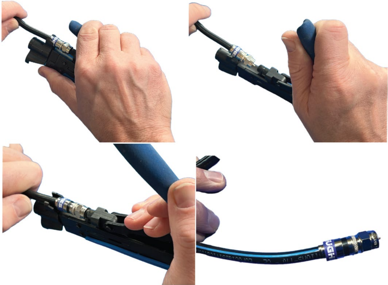
Figure 58: Inserting the IFL cable and connector into the compression tool
