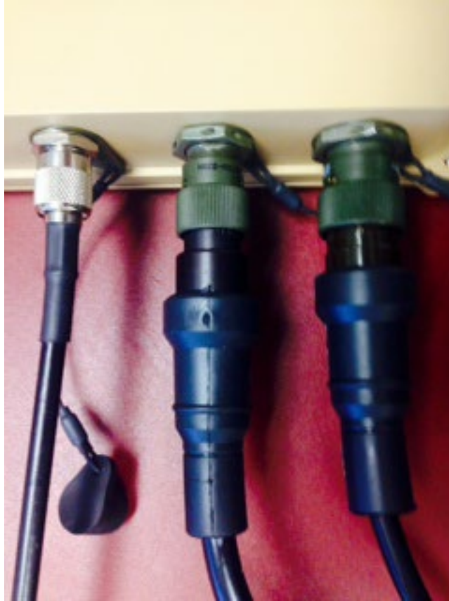
Figure 4-3 Cables Connected: RF, 3-pin and 6-pin respectively
