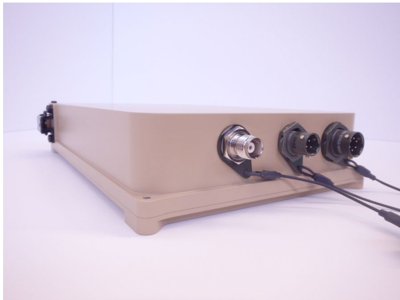
Figure 4-2 Installing Ethernet, Power and RF Cable
