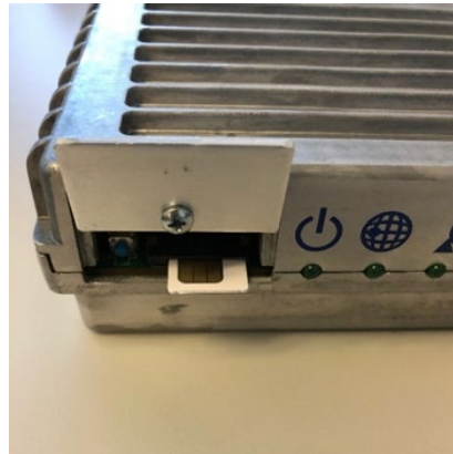
Figure 31: Installing the SIM card
