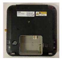
3. Install the battery and completely charge it before using the terminal.
