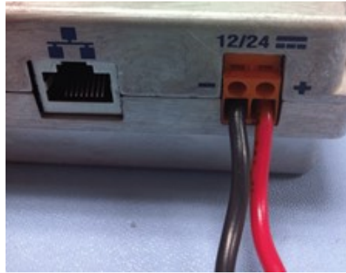
Figure 35: Connecting power leads
