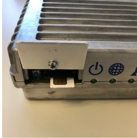
Figure 33: Installing the SIM card
